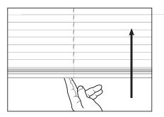
To raise the blind push up from the bottom to the desired height
