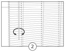
2. Rotate the wand @ clockwise or counterclockwise to open or close the blind slats.
